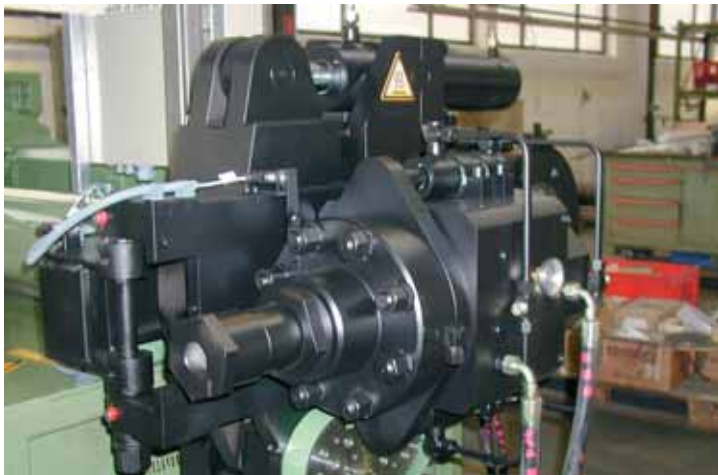
With hydraulic clamping and hydraulic transfer guide ejector
